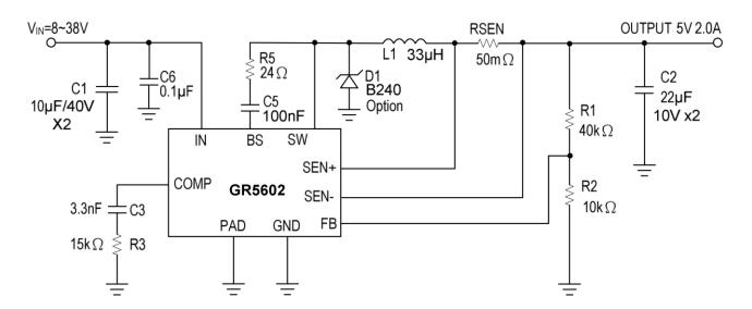
$V_{OUT}=V_{FB} \times (1+R1/R2)$ ,  $V_{FB}=1.00V$ , R2 suggest  $10k\sim30K\Omega$  $I_{SEN} = 2.0A(RSEN=50m\Omega)$
