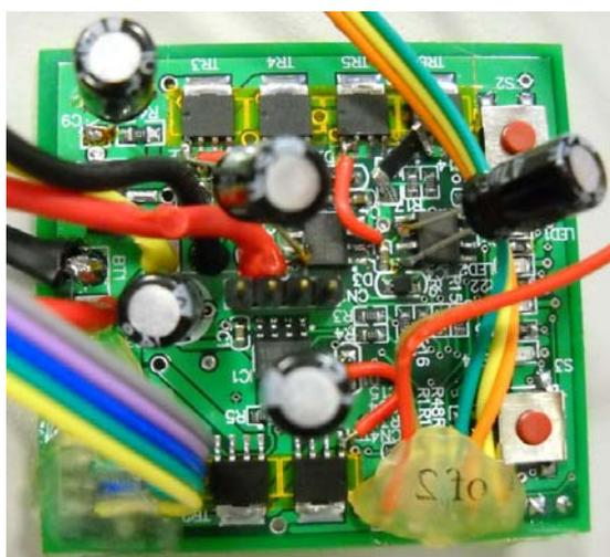
**Figure 6-1 Main board of the controller**
