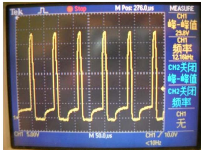
Figure 6-5 Phase driver high side signal
